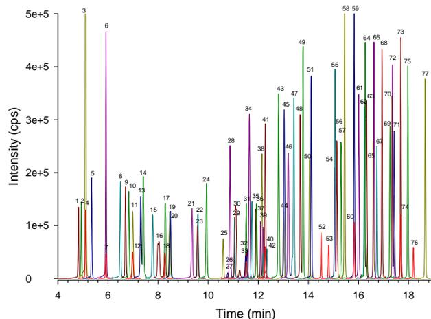
HPLC-MS/MS chromatogram of a calibration curve high point. Overlaid XICs of 77 transitions monitored for 65 compounds and 12 internal standards (internal standards are colored red).
